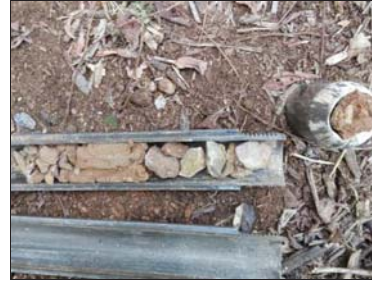
Foto 2: Sondeig S-1, SPT a 1,0 metre.
