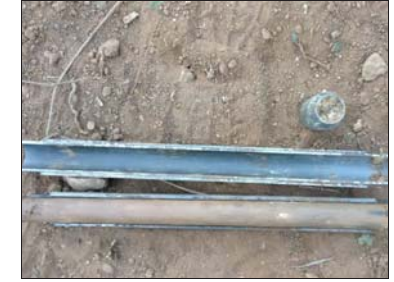
Foto 8: Sondeig S-2, SPT a 6,0 metres.
