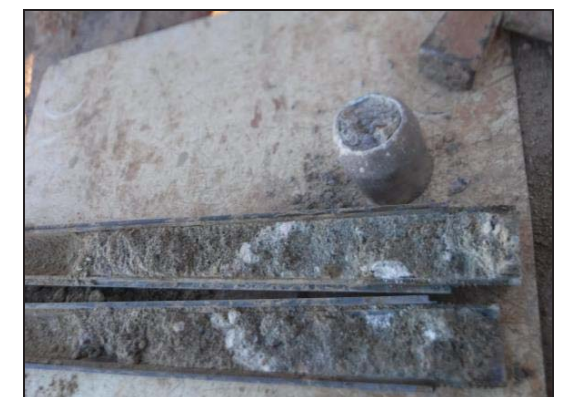
Foto 12: Sondeig S-4, SPT a 1,0 metre.
