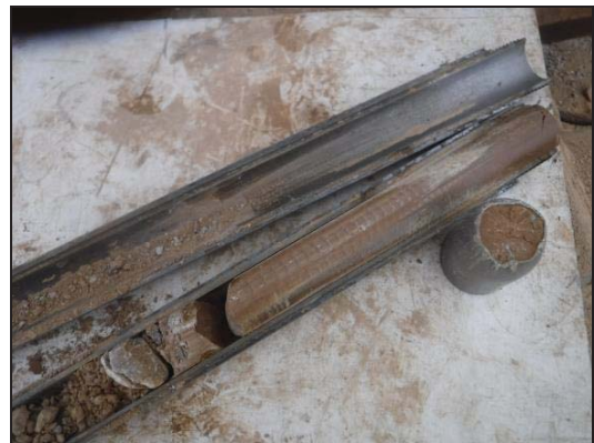
Foto 27: Sondeig S-9, SPT a 2,0 metres.
