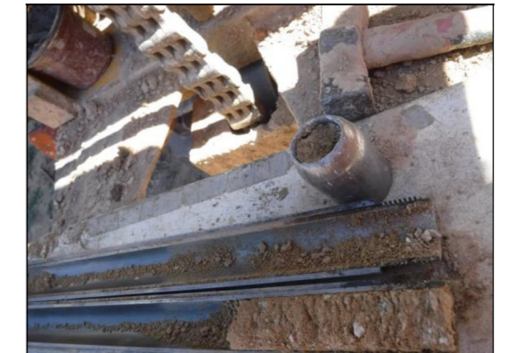
Foto 16: Sondeig S-5, SPT a 4,0 metres.
