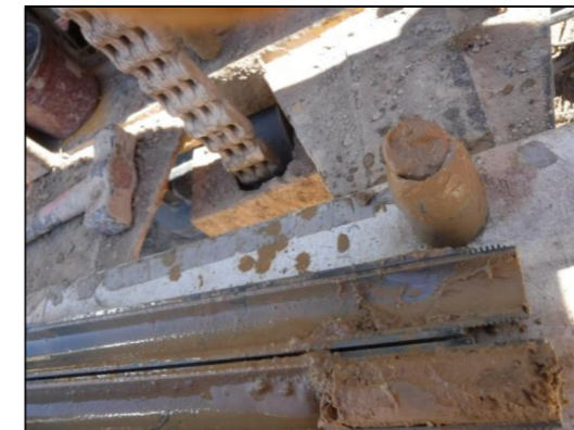
Foto 17: Sondeig S-5, SPT a 7,0 metres.
